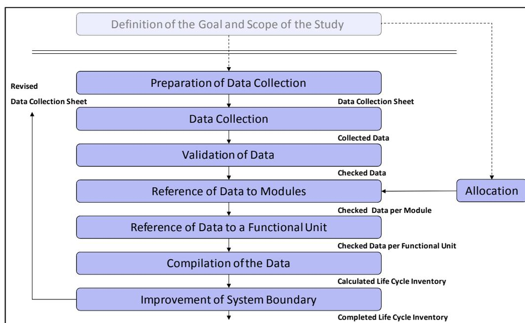
**Figure 13: Simplified procedures for inventory analysis (ISO 2006b) (modified)**
