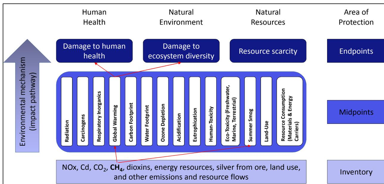
**Figure 11: Schematic steps from Life Cycle Inventory to impact category (JRC 2010a) (modified)**
