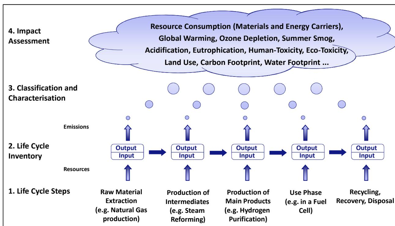
**Figure 1: Overview of the LCA methodology**
