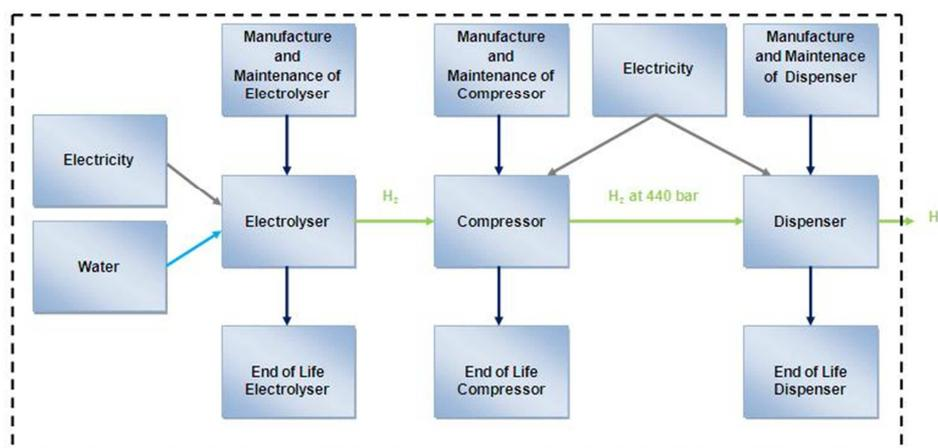
The main processes of this study are the electrolysis, the compression of the hydrogen from 14 to 440 bar @85 temperature) and the dispensing (350 bar @ ambient temperature) of the hydrogen up to the tanking nozzle. For the three main parts the manufacturing, maintenance and end of life processes are also included.
