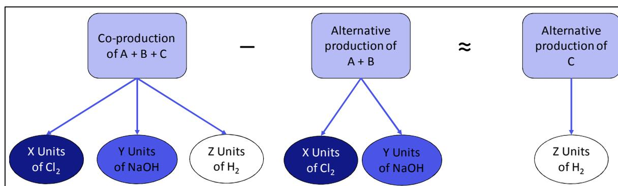
Figure 5: System expansion for solving multi-functionality (JRC 2010a) (modified)
