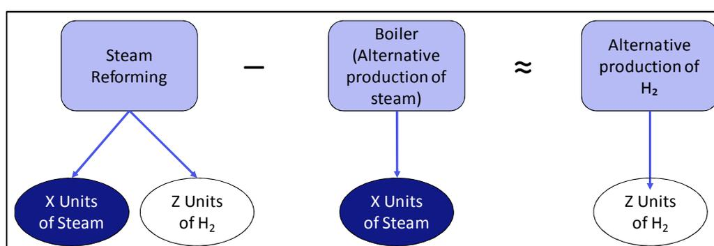
Figure 6: System expansion using the example of a steam reformer
