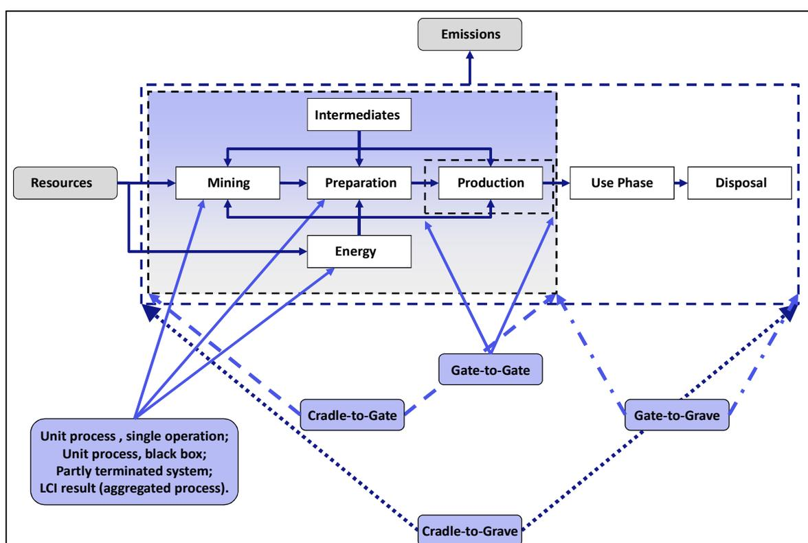
**Figure 9: Possible system boundary in the life cycle**
