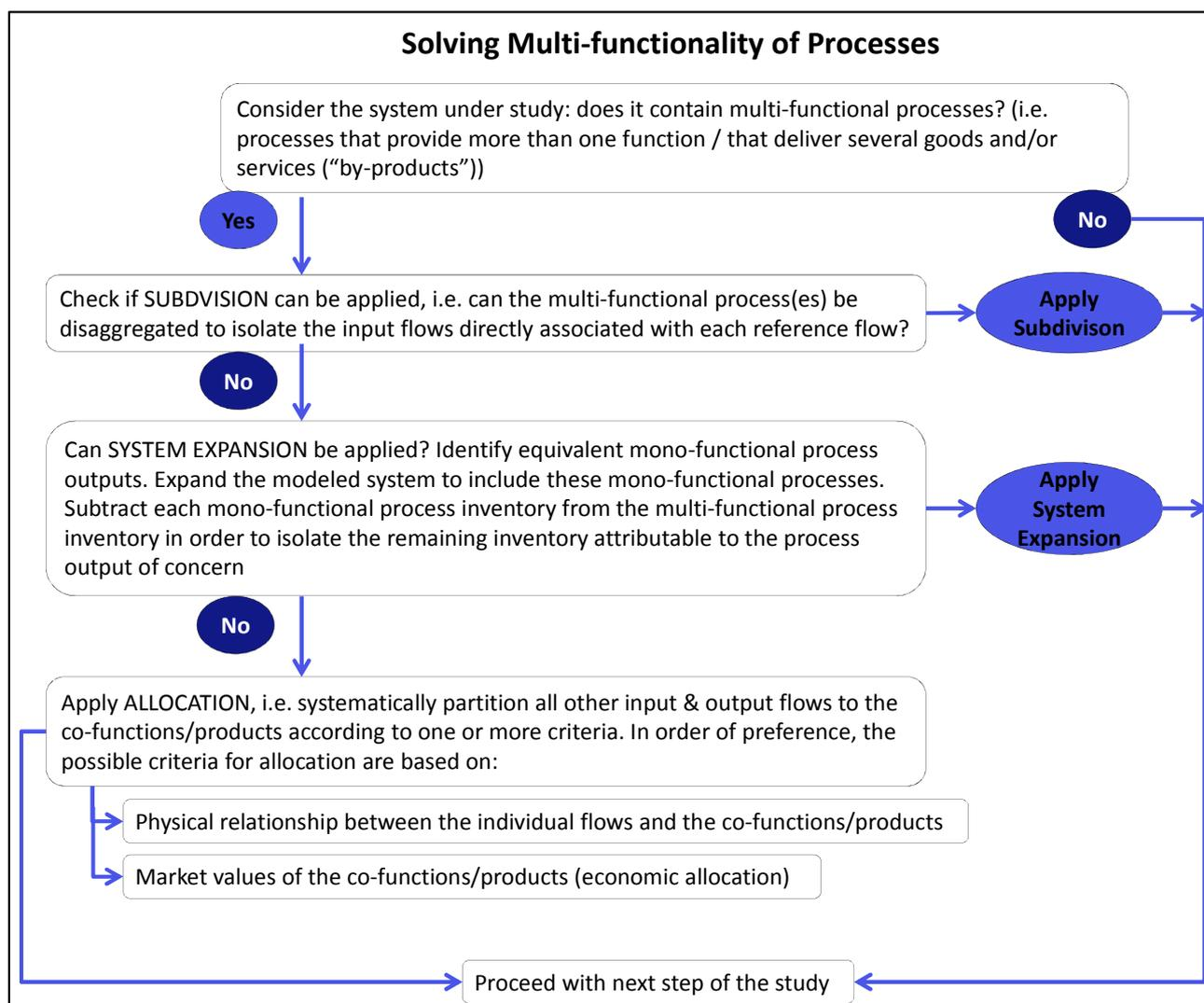
Figure 8: Decision tree for solving multi-functionality provided by JRC-IES (modified)
