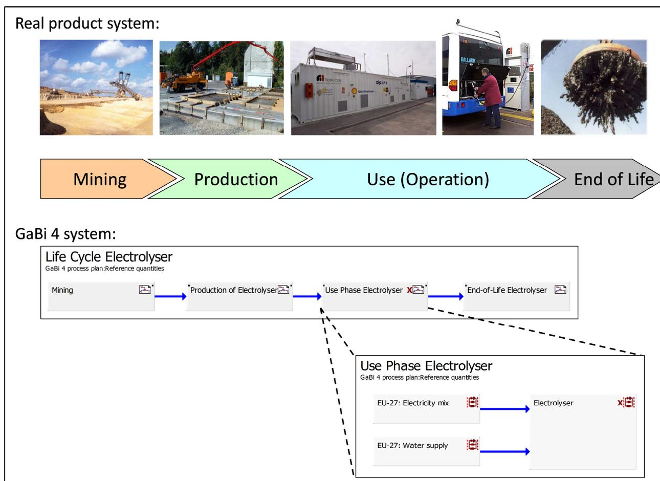
Figure 14: Hierarchical system for real-life modelling in the GaBi software system (LBP, PE 1992-2011) (modified)
