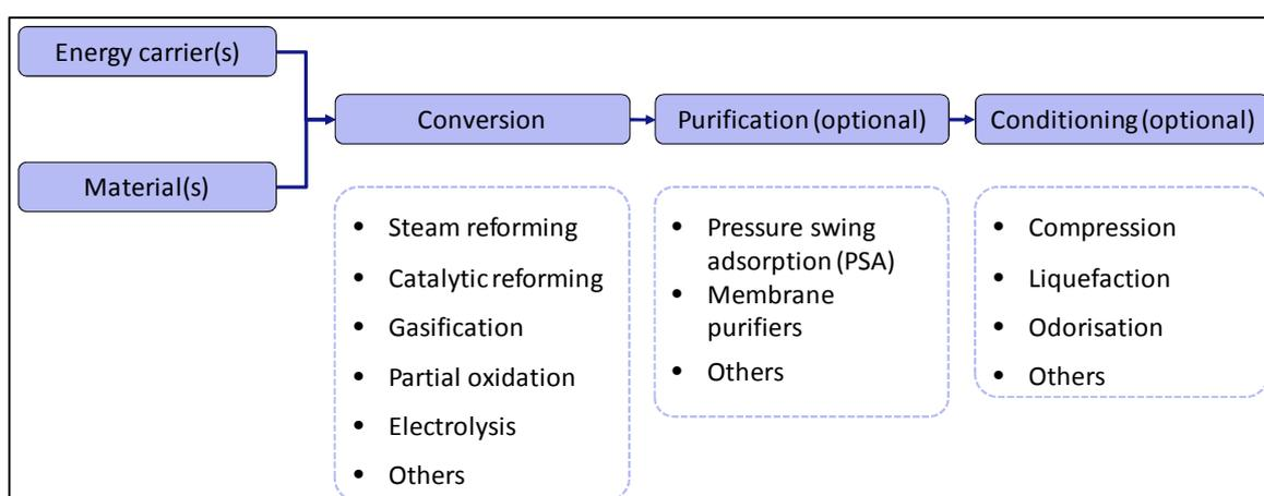
Figure 3: Different pathways of hydrogen production
