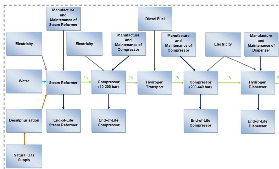
The main processes of this study are the steam reformer, including the desulphurisation of natural gas, the steam reforming itself, the CO-shift conversion and the purification (pressure swing adsorption, PSA) of hydrogen.
